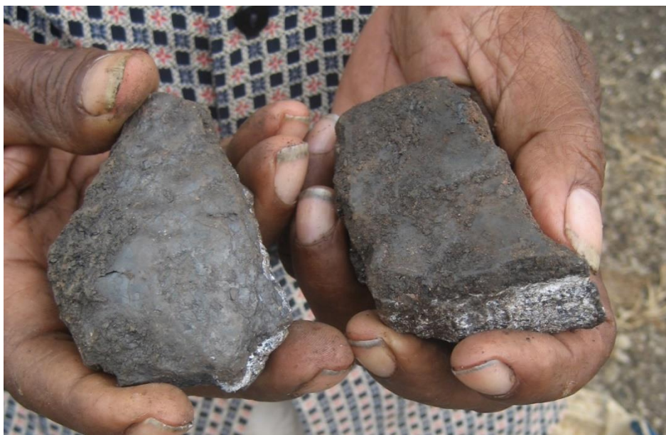
Figure 3. Samples of manganese ore shown to the author in West Timor in 2008. This is only one of several physical forms the mineral takes in West Timor. Photo by author.
